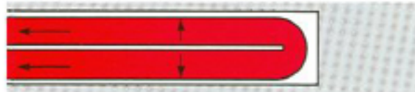
WATT-FLEX HEATER HALVES EXPAND INDEPENDENTLY
