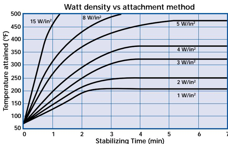
The adjacent graph shows the surface temperature that a silicone rubber heater will attain when suspended in 70° F still air. Below 5w/in<sup>2</sup> watt density applications, the temperature will rise and stabilize at a temperature below the critical 500° F. It is recommended to bond the heater to the surface or even use a pressure plate when the application requires watt densities of above 5w/in<sup>2</sup>.
